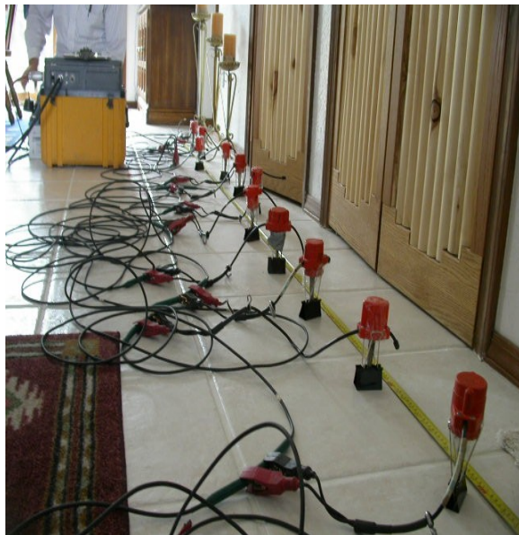
Left: Recording SeisOpt ReMi data inside a house in Arizona, USA done by AMEC Earth & Environmental (courtesy of Mike Rucker). The objective was to analyse soil condition beneath the house. AMEC used 1-ft geophone spacing and the phones were mounted using large binder clips. The noise was induced by shuffling across the floor.
